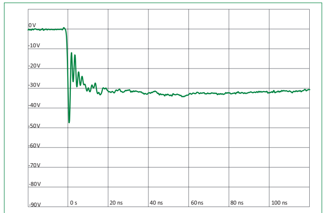
IEC 61000-4-2 -8 kV Contact ESD Clamping Voltage
