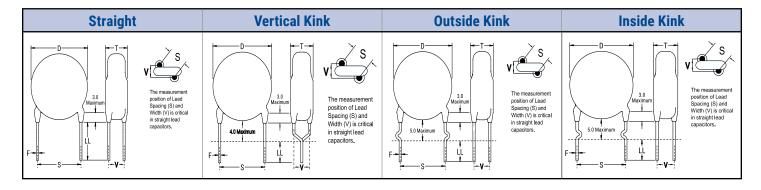
All lead configurations are available on devices with lead spacing of 10 mm and 12.5 mm.
